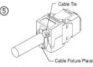
Fasten a cable tie wrap to secure the cable fixture place.
