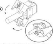
Secure the hinged outlet by using a crimp tool until it completely snap to effect the connection.
