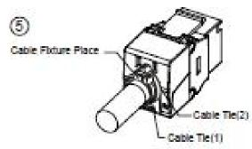
Fasten cable tie(1) to secure the grounding. Optional cable tie(2) for securing of flaps.
