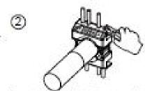
Insert a cable into the termination cap and fan out all four twisted pairs. Following the instruction of the colorcoded wire position printed on the termination cap, position conductors into the slots and make sure the conductors are in the proper slot. Trim the ends of the conductors
