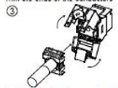
Install the termination cap to outlet, which will also allocate the conductors sitting on the slots.
