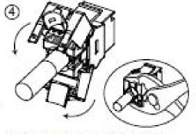
Secure the hinged outlet by using a crimp tool until it completely snap to effect the connection.
