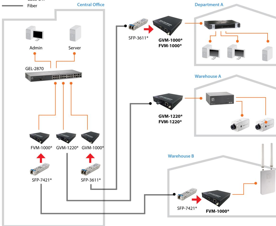
\*In above example diagram, converter modules at local and remote ends should be paired for proper connectivity, and the distance mainly depends on cable and transceiver selection accordingly.
