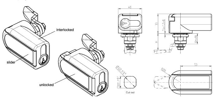
Profile half cylinder DIN 18252 (EN1303) dimension A=30 equals total length 40. The locking cam has to be between 3 and 5 o'clock.
