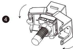
Push the termination cap down by closing the wing covers
