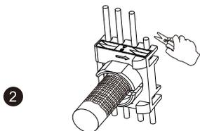
Insert the cable through the termination cap, untwist the four pairs and fan out. Following the colour code on the cap, insert the wires into their designated slots. Double check the wires are in the correct positions and then trim off the excess.
