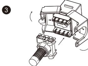
Position the termination cap on the keystone IDCs follow the correct orientation
