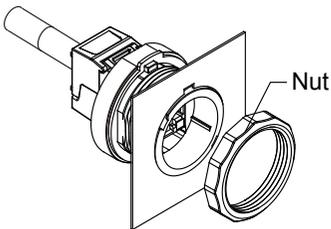
3. Screw on the nut to complete installation.
