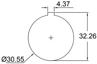
Recommended cutting on panel , panel thickness 0.7 ~ 2.0mm
