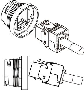
1. Finish the installation of Keystone Jack first. Place the Keystone Jack with latch side aligned to “↑” on the IP68 socket housing, snap the Keystone Jack into IP68 socket housing
