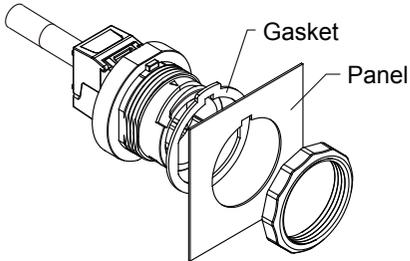
2. Place the IP68 socket housing to panel. Make sure to place the gasket in between panel and housing properly.
