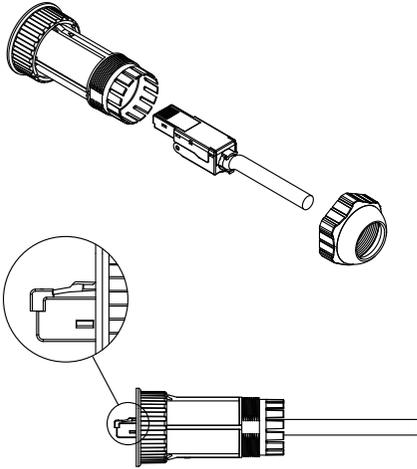
2. Ensure the latch on plug placed on the right position to the IP68 housing and locked properly inside the housing.
