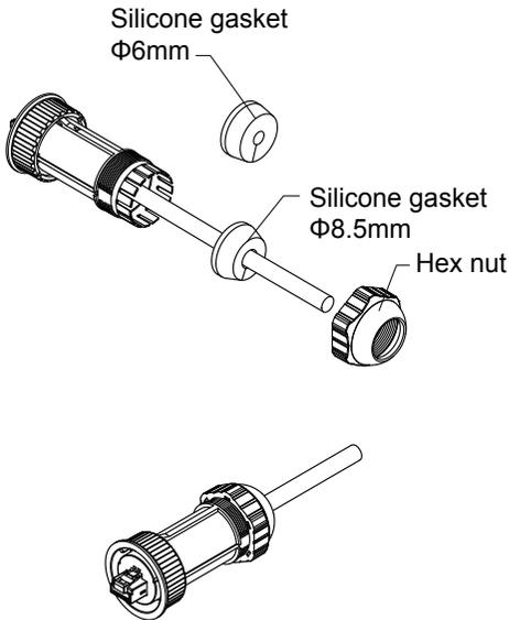
3. Place the silicon gasket and screw on the Hex Nut tightly to ensure the watertight function. Using a hex wrench to help when necessary.
