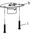
Use a stud finder to locate the stud. It is a good idea to verify where the stud is located with an awl or thin nail. Pre-drill a 50mm deep hole at the stud using a 3.8mm drill bit. Make sure the hole is in the center area of the stud. Use the Wall Plate(b) as a template to mark the location of the second hole in the stud. Drill 50mm deep hole using the 3.8mm drill bit in the marked location. Attach the wall plate to the wall using the 2 pieces Lag Bolts(l).
