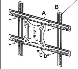
Install the "B" to back of TV first before connect to the "A".
