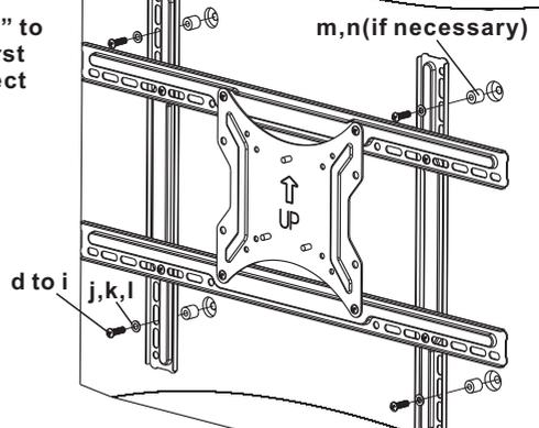
First of all, make sure the diameter and length of the Bolt(d,e,f,g,h,i) your TV requires. Once you have determined the correct diameter and length, you will thread the Bolt into the TV using the correct Washer(j,k,l). Use the Spacer(m,n) only if the bolts are too longer.
