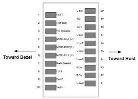
**Pinout of Connector Block on Host Board**
