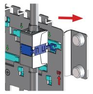
Put the coupler in the provided opening. Slide it down until the plastic latch locks.
