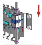
Secure the coupler housing and shield contact via cable tie. Fix the cable to the strain relief via cable tie.
